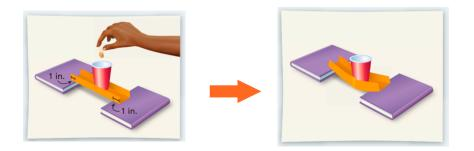
• Put two *new* strips of paper together to make a bridge with twice as many layers. Find the breaking weight for this bridge.
